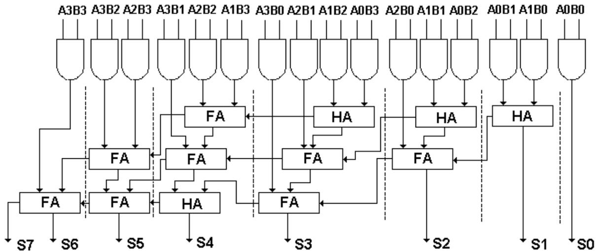
The first level of 16 AND gates computes the individual partial products. The second- and third-level logic blocks form the accumulation of the products on a column-by-column basis. The column sums are formed by a mixture of cascaded half adders (HA) and full adders (FA). In the figure, inputs from the top are the bits to be added and the input from the right is the carry-in. The output from the bottom is the sum and to the left is the carry-out.
